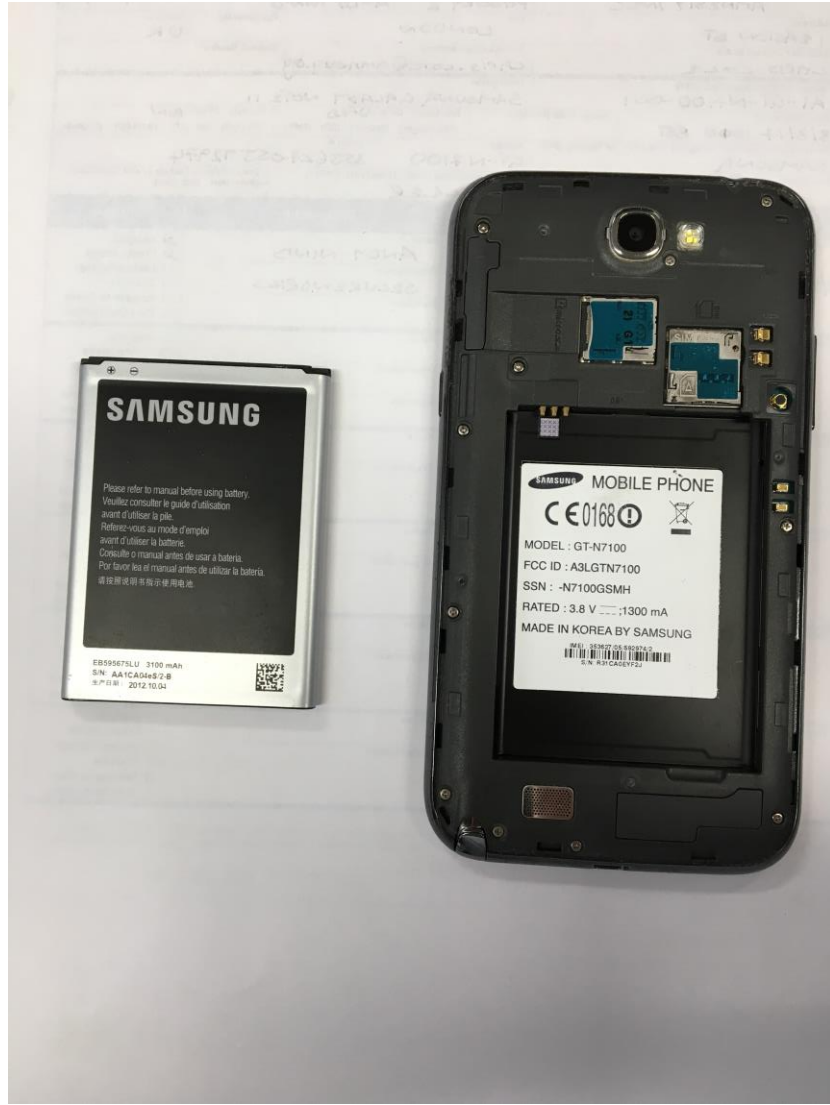
Figure 2 – Internal back view with battery removed
