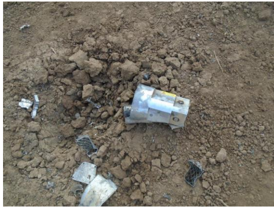
Fig.3 Scrap from the GBU-69/B, including the distinctive mesh tail fins in the crater. © SOMALIMEMO
